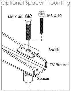
Spacer is used when the back of TV is not flat or the mount holes are sunk into the back of the TV. (Rarely used)
