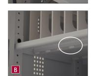
try a flat-head screwdriver. To install the divider, angle the divider into a slot at the back of the shelf, then tilt the divider into place at the front of the shelf. Label each bay with the bay numbers. [Image B]
