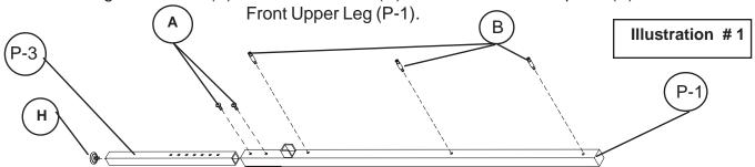
3.) Screw in a Glide (H) into the bottom of one Insert Leg (P-4). Place the Insert Leg (P-4) into the bottom of the Center Back Upper Leg (P-2) and secure at the same height as the Front Leg using two Screws (A) as shown in illustration #2. Tighten Screws (A) with Allen Wrench (C). Screw in nine Camposts (B) into the Center Back Upper Leg (P-2).
