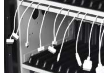
Cords are held in place with protective foam.
