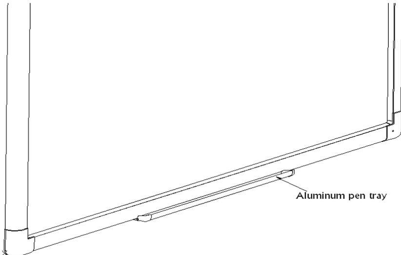
Grey color frame with pen tray: In the frame of the board, prior to securing the pen tray you will find a slot that accommodates a Kensington lock. If you would like to use a Kensington lock insert and loop the cable through the center hole on the frame, position the pen tray in line with the four screws, and then screw the pen tray in place. (Shown below)
