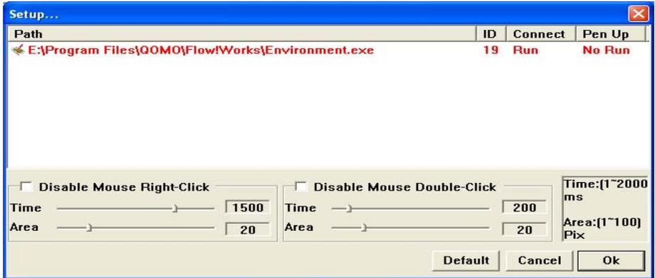
System setup is used to set the simulation of mouse's right-click and double-click based on user's preferences.
