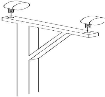
(2) With an assistant's help, hang Interactive whiteboard on the floor stand by lowering the two bolts onto the top hooks and securing the bottom bolts into the bottom hooks. There are two heights for hanging according to user's preferences. (as shown below)
