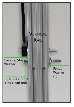
Step 5: Put (1) Locking Star Washer on each of the 1/4 -20 x 3.50 Hex Head Bolts.
