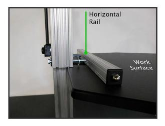
Step 8: Lift the Work Surface up and align the holes in the Horizontal Rail with the (2) 1/4-20 x 3.50 Hex Head Bolts. Push the Work Surface onto the Hex Head Bolts until the threads of the bolts come through the Horizontal Rail.
