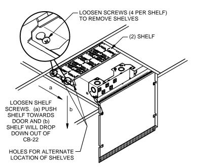
4b. FOR 1RU x 19" EIA RACK-SIZED ELECTRONICS, INSTALL RACK MOUNT BRACKETS AS SHOWN. INSTALL RACK UNIT AND RE-INSTALL SHELF INTO CB-22. MAKE ELECTRICAL CONNECTIONS AS REQUIRED.
