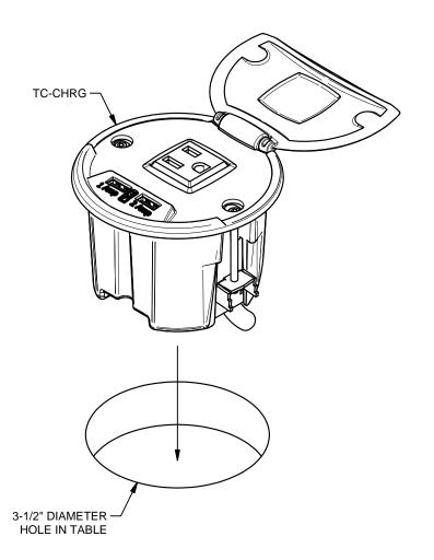
2. SECURE TC-CHRG ASSEMBLY TO TABLE BY TIGHTENING MOUNTING SCREWS. ALTERNATELY TIGHTEN LEFT AND RIGHT SCREWS TO MAINTAIN CENTERING OF ASSEMBLY IN TABLE.
