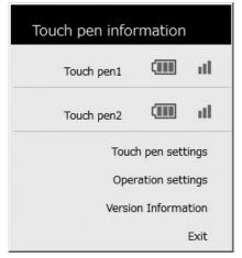
Touch pen information: Shows the registration number, the battery level and the signal strength of the active pen being
