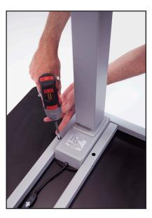
For narrow frame models (42", 47" and 59"), connect the frame and desk at 12 points with the 12 screws provided (Part # 12). For wide frame models (71" and 83"), connect the frame and desk at 14 points with the 14 screws provided (Part # 12). The 2 extra screws are to be used to connect the metal sleeve through the extension channel into the underside of the desk.
