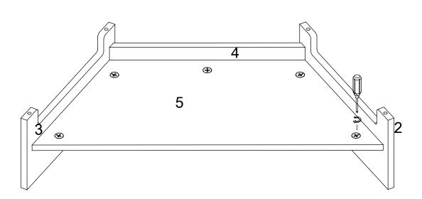
Turn Cam Locks on Part 5 one-half rotation clockwise to complete the connection. Do not over tighten
