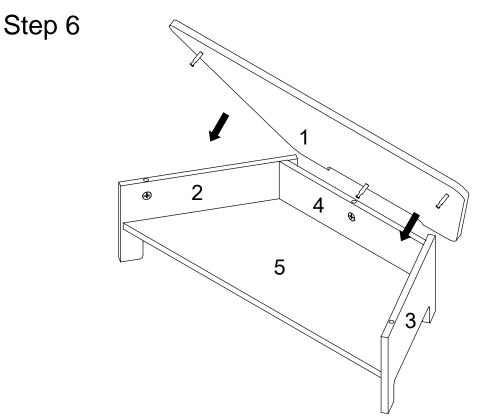
Flip the assembly right-side up. Attach Part 1 to Parts 2, 3, and 4. The Dowels from Part 1 go into the top access holes of Parts 2, 3, and 4.
