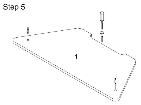
Use Screwdriver to insert Dowels into small white threaded holes on Part 1.
