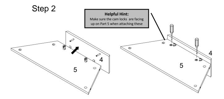
Attach Part 4 to Part 5. The two Dowels on Part 4 go into the two side access holes on Part 5. Turn Cams on Part 5 one-half rotation clockwise to connect 4 and 5 together. Do not over tighten.
