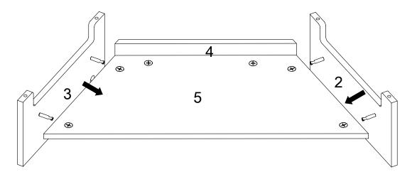
Attach Parts 2 and 3 to Part 5. The two Dowels on Part 2 go into the side access holes on Part 5. The two Dowels on Part 3 go into the other side access holes on Part 5.
