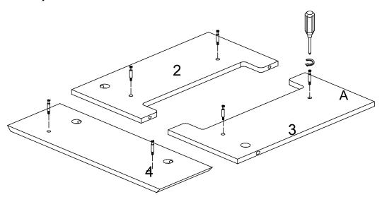
Use Screwdriver to insert Dowels into small white threaded holes on Parts 2, 3, and 4. Insertion should be easy. If strong force is required, back out the Dowel and start again. Turn Dowel until all threads are no longer visible.
