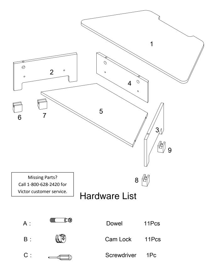
This product uses a system of Dowels and Cam Locks to connect pieces together.
