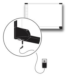
3 Connect the TS 600 Bluetooth adapter to the serial port on the whiteboard.
