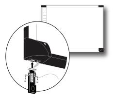
4 Use a screwdriver to install and tighten the two screws supplied for the adapter.
