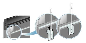
2 Slide the whiteboard carefully to align the safety straps with the holes in the top of the whiteboard.
