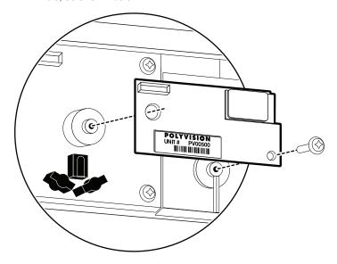
6 Secure the WT Bluetooth adapter using the screw provided.
