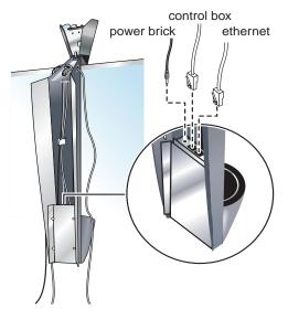
4 Secure the cables to the body of the camera arm (for strain relief) using the cable ties inside the arm.
