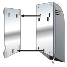
Removing the Control Pad From its Mounting Plate
