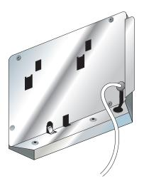
7 Route the RJ14 cable from the back of the control pad into the wall and up to the camera arm mounting plate exit hole. If necessary use a fish tape to fish the cable end through the wall to the camera arm mounting plate exit hole.
