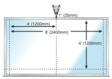
Position the four corner calibration sheets within the 4' x 8' (1200mm x 2400mm) limit as shown below. If your board is
