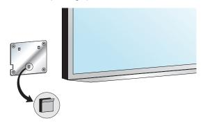
3 Drive the toggle bolt screws (provided) through the mounting plate and toggle bolt, and if a stud was located, drive a #8 x 1.5" (38mm) drywall screw (provided) through the mounting plate and wall into the stud.
