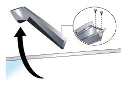
3 Fasten the arm in place using the two arm-securing thumb screws provided.
