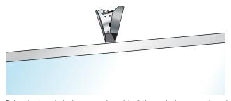
3 Drive the toggle bolt screws (provided) through the mounting plate and toggle bolt, and if a stud was located, drive a #8 x 1.5" (38mm) drywall screw (provided) through the mounting plate and wall into the stud.
