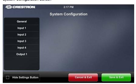
The **System Configuration** screen contains buttons to select specific setup screens. There is a **General** entry, plus an entry for each input and output.
