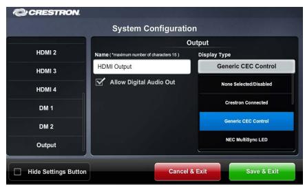
Use the Name text box to enter the output name you want to display on the main screen.
