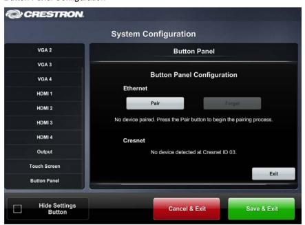
4. Tap Pair to begin the pairing process. All the LEDs on the MP-B10 will blink. (On units with older firmware, only one LED will blink.)
