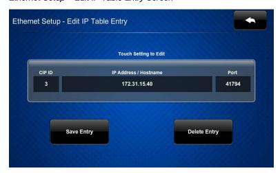
3. Tap the CIP ID field to display the on-screen hex keypad.
