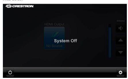
Tap the (gear) icon to the right of the (power) button to display the **System**Configuration screen. If the gear icon is not visible on the main screen, touch and hold the bottom right corner of the screen for 10 seconds to display the **System Configuration** screen.
