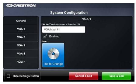
Use the **Name** text box to enter the input name you want to display on the source selection screen (shown on page 22).
