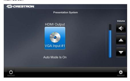
The right side of the main screen contains the volume controls and a volume gauge to provide visual indication of the volume setting.
