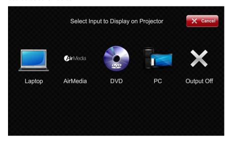
All enabled inputs are shown on this screen. Tap an input to route its video to the output while the associated audio is routed to the analog audio output.
