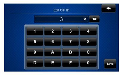
4. Use the keypad to make the new entry. Tap **Save** to save the new entry or to return to the **Ethernet Setup – Edit IP Table Entry** screen.
